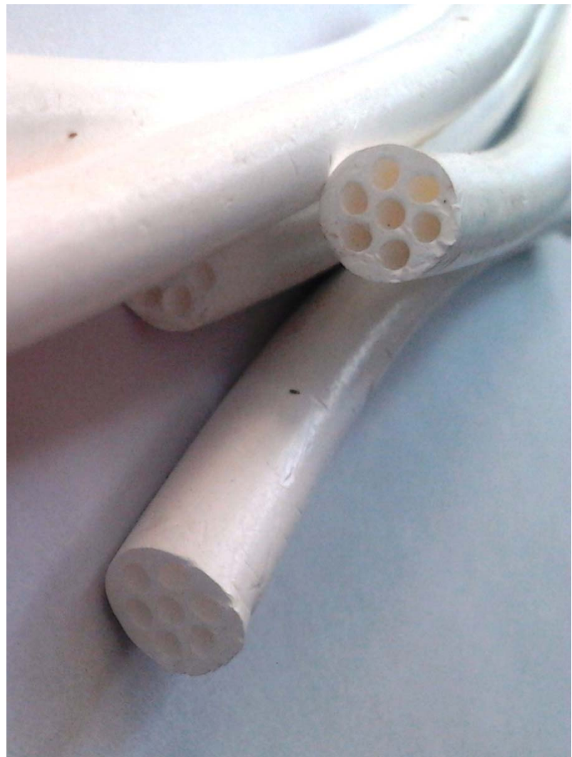
Multi-bore hydrophilic ultrafiltration membrane used on non-modular unit has self-supporting system
